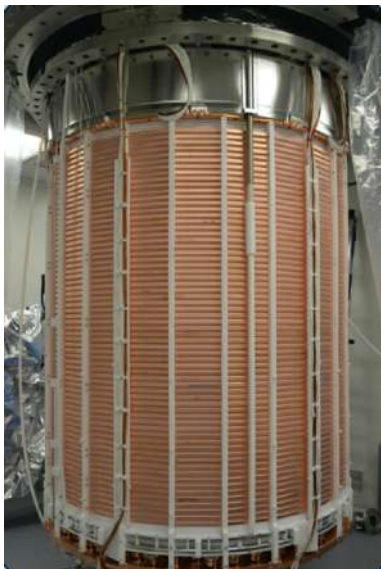
TPC installed underground
